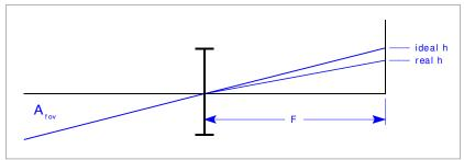
The height t of the point "ideal h" is F tan (A). The height of the point "real h" is different. Such a lens is said to have distortion.
