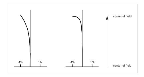
Both lenses have about 1% distortion, a value that is normally acceptable, even in visual instruments like cameras.
