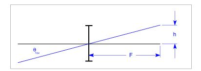
In an ideal lens, there is no distortion, and the height of a point on the image is simply:
